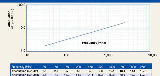
Calculate Attenuation = (0.300717) • FMHz + (0.000335) • FMHz (interactive calculator available at http://www.timesmicrowave.com/cable\_calculators) Attenuation: VSWR=1.0 ; Ambient = +25°C (77°F) Power: VSWR=1.0; Ambient =  $\sqrt{40°C}$ ; Inner Conductor = 100°C (212°F); Sea Level; dry air; atmospheric pressure; no solar loading
