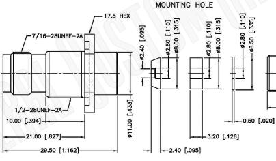
1. CRIMPED CONTACT PIN HEX CRIMP SIZE .068"
