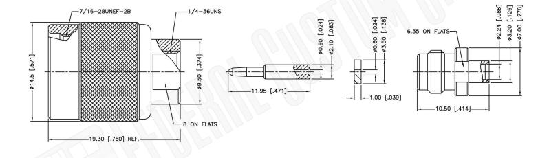
NOTE: 1. CRIMPED CONTACT PIN HEX CRIMP SIZE .068"
