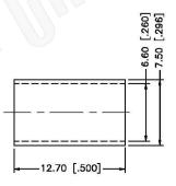
CRIMP NOTES: 1. CRIMPED FERRULE HEX CRIMP SIZE .255" 2. CRIMPED CONTACT PIN
